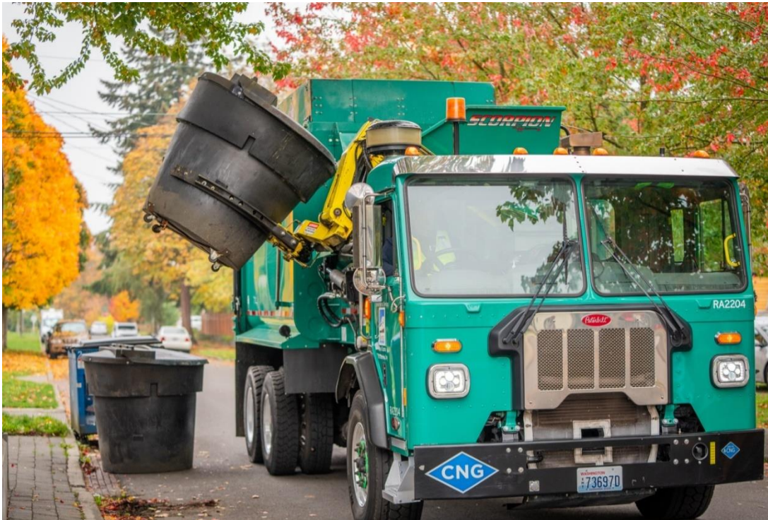
SWM Vehicle servicing 300-gallon automated collection container
